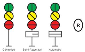
Signal post replacement switches (SPRS) are provided at some automatic and semi automatic signals. When operated they place the signal to danger, if this is the case, then on the signal diagram it will specify with an "R" identifying the signal to have an SPRS.
