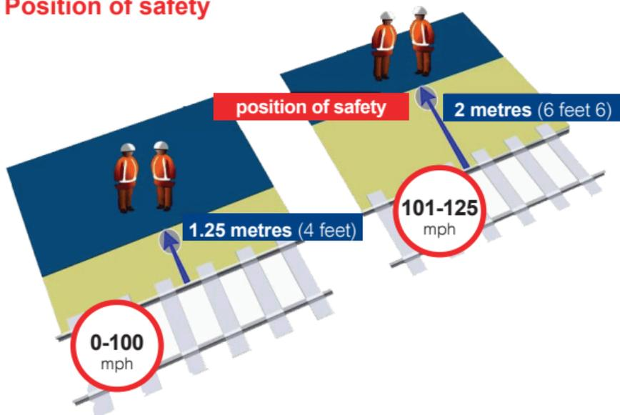
Lightweight tools and equipment must be left at least 2 metres (6 feet 6 inches) from the line, irrespective of the speed limit.
