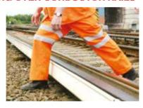
If you need to step over the conductor rail and adjacent running rail you must do so in one step, preferably where the ballast is level and where there is either timber or plastic guard boarding present. Never step between the conductor rail and adjacent running rail.
