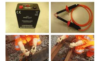
After your COSS has been issued with a conductor rail permit the conductor rail(s) must be tested at the site of work immediately prior to the commencement of work.
